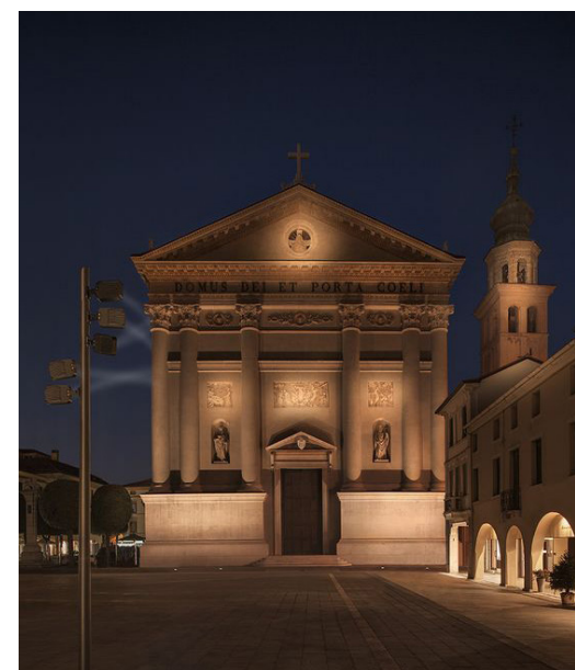
Spotlights mounted to smart poles to light onto select heritage façades. Luminaire selection have narrow beam/ asymmetric lens optics to highlight key features of buildings.
