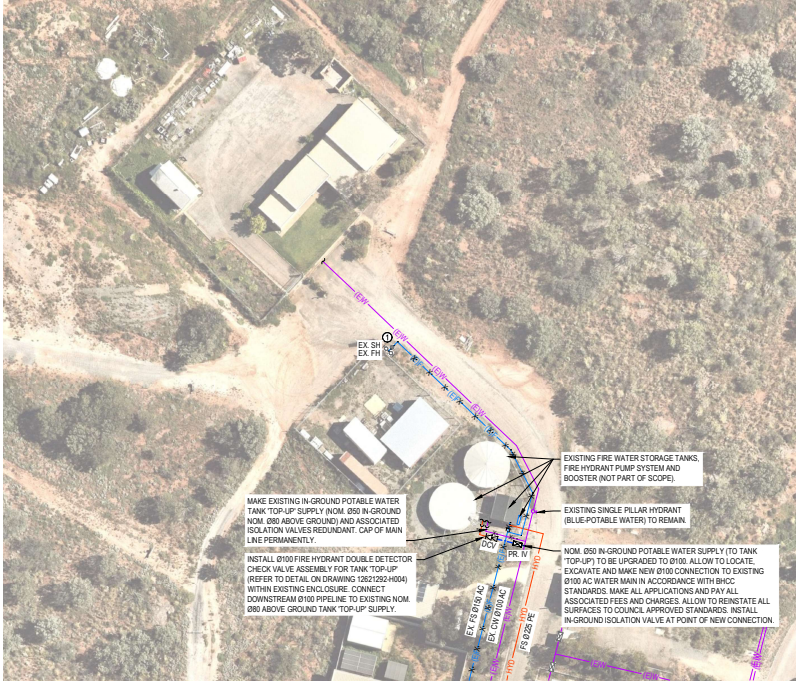
FIRE HYDRANT SYSTEM DESIGN SHEET 3 OF 3 SCALE 1:500
