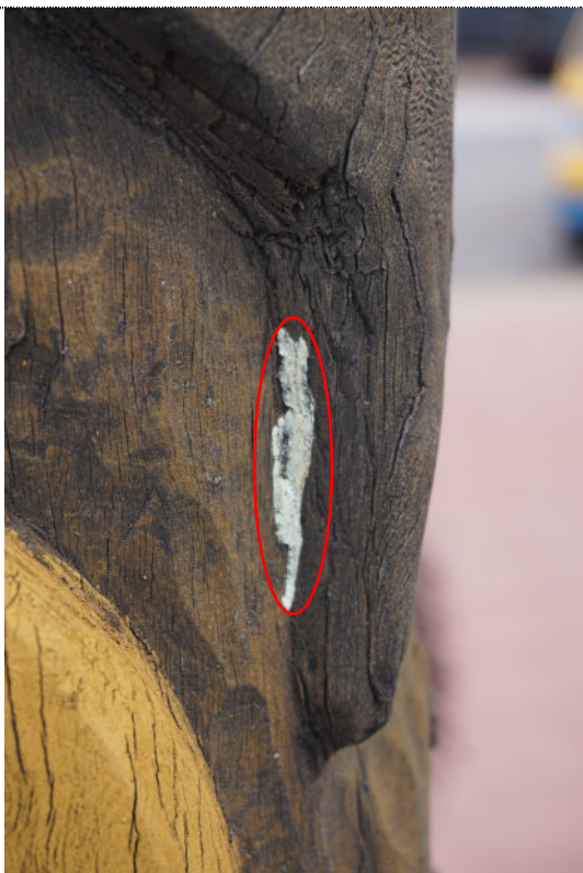
Figure 86: Detail – Pole #2003.0023, Untitled , exterior, UV degradation (darkening) to wood surface throughout. Surface dirt and insect debris noted throughout, including the presence of bird excrement (highlighted in red).
