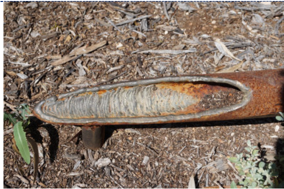
Figure 6: Detail – dirt particulate within tube; surface corrosion.
