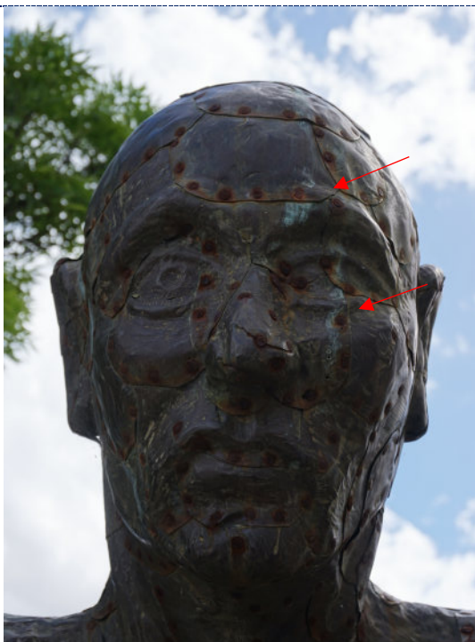
Figure 15: Detail – exterior, isolated surface corrosion products; corroded iron nail heads.
