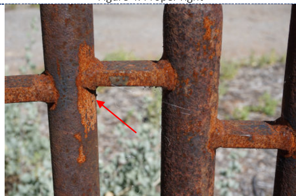
Figure 6: Detail – dirt particulate; surface flash rusting at new welds created during manufacture of artwork.
