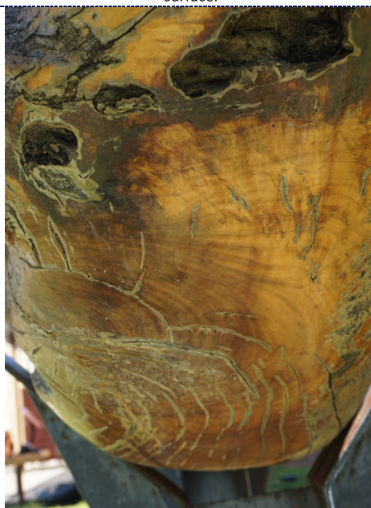
Figure 18: Detail – exterior-bottom, degraded and peeling varnish.
