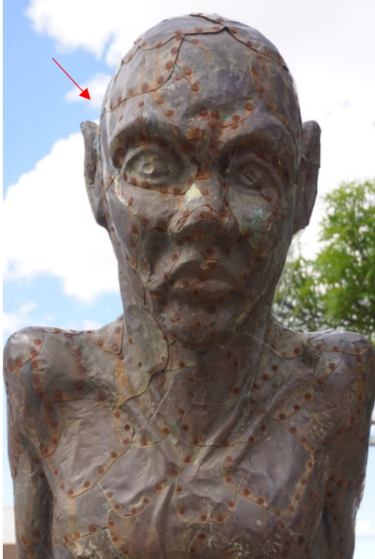
Figure 7: Detail – exterior, isolated surface corrosion products; corroded iron nail heads; bird excrement (arrow).
