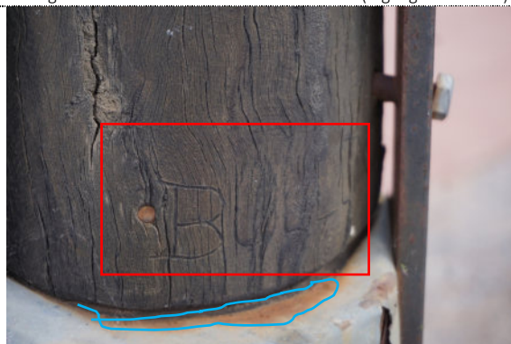
Figure 144: Detail – Pole #2003.0028, Emu and kangaroo tracks , exterior, UV degradation (darkening) to wood surface throughout. A large accretion noted on the wood surface (highlighted in red).
