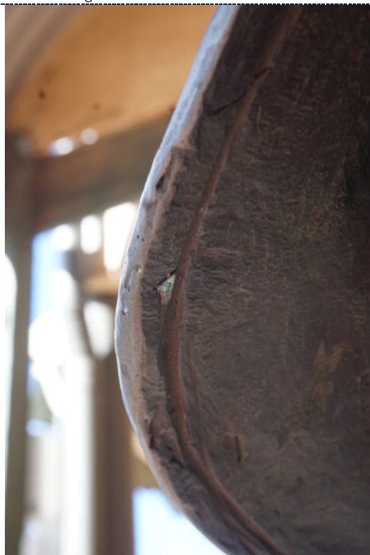
Figure 14: Detail – corrosion product inside small casting defect.
