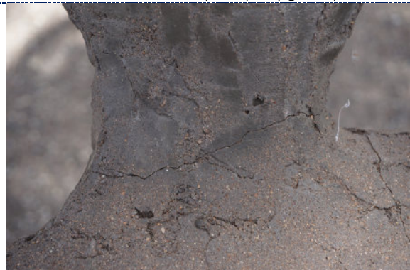
Figure 12: Figure 1 – Detail – dirt particulate, surface cracks.
