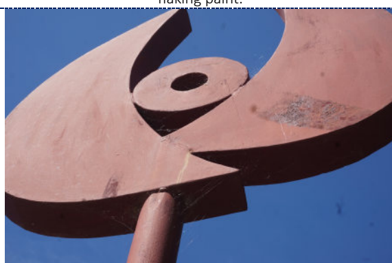
Figure 9: Detail – paint chalking, flaking paint loss with overpaint; dirt particulates and spider webs.
