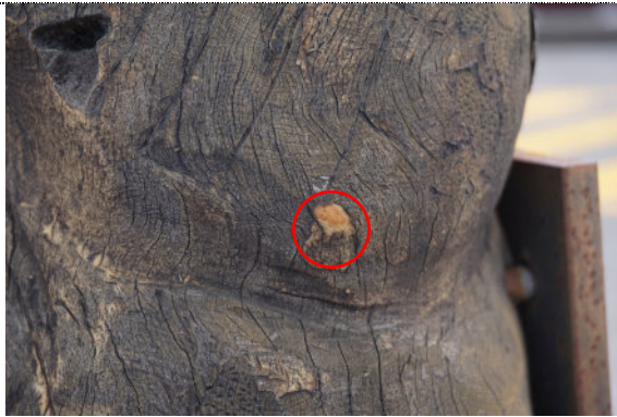
Figure 98: Detail – Pole #2003.0024, Untitled , exterior, exterior, UV degradation (darkening) to wood surface throughout. Small yellow accretion affixed to the exterior side of the pole (highlighted in red).
