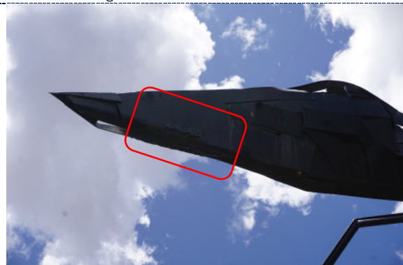
Figure 8: Detail – paint loss and corrosion to iron substrate.
