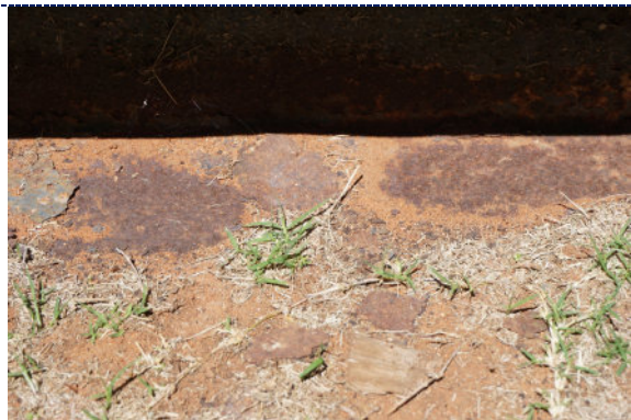
Figure 24: Detail – corrosion product on the ground stemming from the canoe mount.
